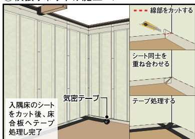
④横張り吊り下げ施工-4
